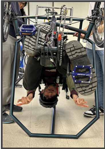
Figure: The rider suspended by the vehicle while the vehicle rests upside down.
